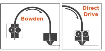
in a **Bowden** system, but the trade-off is it tends to make the print head heavier, meaning it can't move quite as fast as a **Bowden** can. **Bowden** systems mount the gearing which applies the force somewher on the printer frame, and it is fed through a line of PTFE tubing to reach the hotend.
