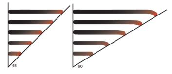
**Overhangs and Support** are directly related. An overhang is when a printed layer lies outside of the layer beneath it - a general rule of thumb for overhangs is that they're fine up to 45 degress, and anything over 60 degrees definitely requires a support structure. The 15 degrees in between can vary from material to material, but Cura is fairly good at guessing this.
