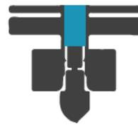
Significant gap can create backpressure and overflow issues out of the heat block.
