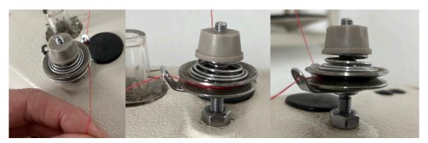
Bring the thread through the back hole of the bobbin tensioner, between the tension discs, then through the 2nd hole on the left of the tensioner. This tension knob can be adjusted if the bobbin is not winding securely and smoothly. Make small adjustments though!
