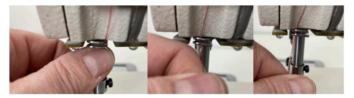
Wind the thread through the spiral so it goes through the center of the spiral holder as above
