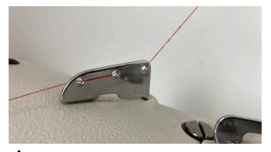
Bring the thread up from the cone and through a hole in the T post back to front (not pictured). Then, wind the thread through the 3 hole guide.
